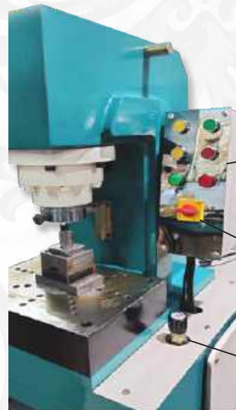
Die Fitting and Working Area
